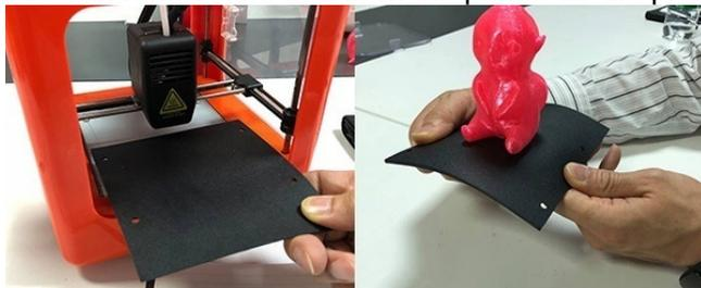
**4.5 Retract:** If want to replace another roll of filament or the machine does not print for long time then needs to retract the filament. First shift the gear to "RETRACT gear, the light inside print button will flash, And **Please be patient and wait a few minutes,** Motor begins to work, use hand to pull the material until it completely retract from the tube. then shift the gear back to middle position.
