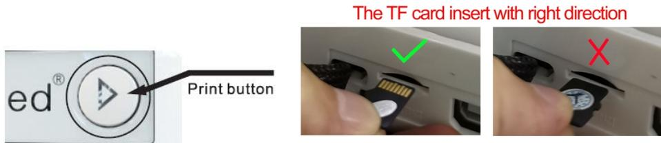
● Insert the TF card to the printer (**insert with right direction**), and press the print button, the printer will automatically warm up, and the light will flash.
