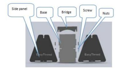
(2)Put the Nuts insert into the slot of base, to Insert M3 screw from the side panel. Fasten the side panels and base, then get bridge through the center hole of filament holder, then finally to put the bridge insert the side panels.
